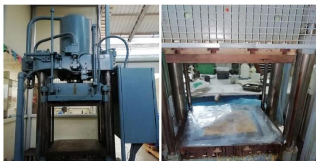
(a) Compression molding setup (b) Fiber arrangement in mold
