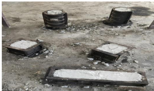
Fig 5 Casting of concrete specimens
