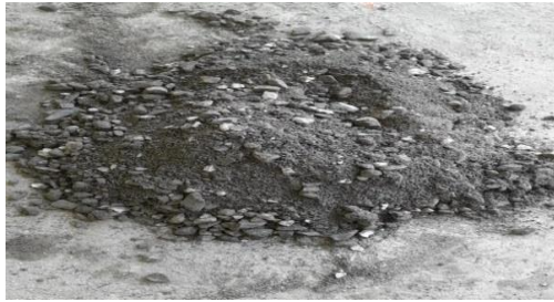
Fig 4 Mixing of concrete specimens
