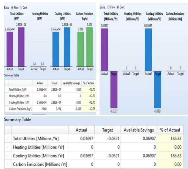
Fig. 7: ASPEN software output indicating Energy saved on major utilities duty flow mainly between target and actual values for MEA treatment plant.
