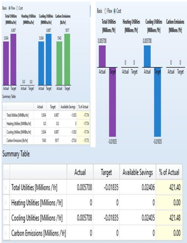
Fig. 4: ASPEN software output indicating Energy saved on major utilities duty flow mainly between target and actual values for MDEA treatment plant.
