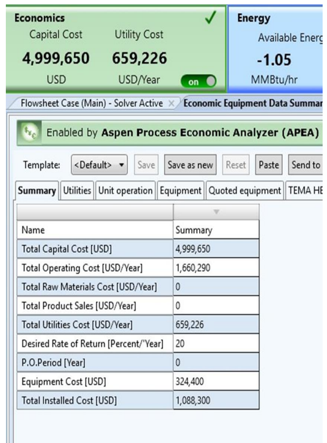
Fig. 3: Overall summary of the economic analysis result using MDEA as a solvent in an acid gas treatment plant from the Aspen Process Economic Analyzer (APEA) software.
