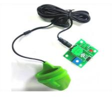
A heart rate monitor (HRM) is a personal monitoring device that allows one to measure/display heart rate in real time or record the heart rate for later study. It is largely used to gather heart rate data while performing various types of physical exercise.
