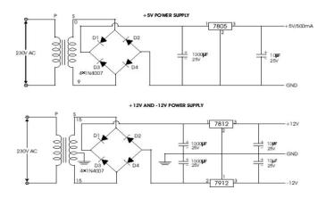
A fixed three-terminal voltage regulator has an unregulated dc input voltage, Vi, applied to one input terminal, a regulated dc output voltage, Vo, from a second terminal, with the third terminal connected to ground. The series 78 regulators provide fixed positive regulated voltages from 5 to 24 volts. Similarly, the series 79 regulators provide fixed negative regulated voltages from 5 to 24 volts.
