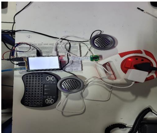
Figure.2 face recognition smart attendance system hardware model
