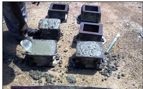
Fig.1 Casting of cube
