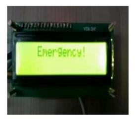
The LCD display can exhibit the text message when controlled by an Arduino-equipped smart glove is shown in the above fig. By utilizing a combination of temperature sensor, pressure sensor, and accelerometer with an Arduino UNO, the body's position, air pressure, and temperature can be accurately identified is shown in the above fig.
