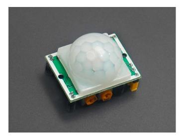
A PIR (Passive Infrared) motion sensor is a device that detects motion by measuring changes in infrared radiation emitted by objects within its field of view. These sensors are commonly used in various applications, including security systems, automatic lighting, and occupancy detection.
