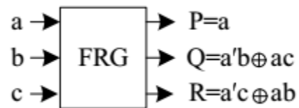
Figure 5: Block diagram of Fredkin gate
