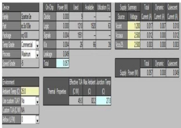
Figure 9: Power Analysis of Viterbi encoder
