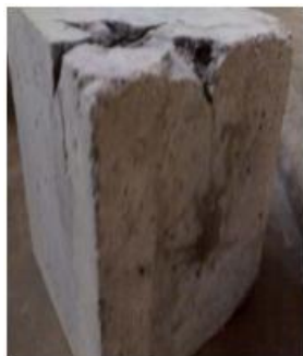
Figure crack pattern in Cube
