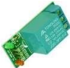
Fig.6 Single Channel Relays
