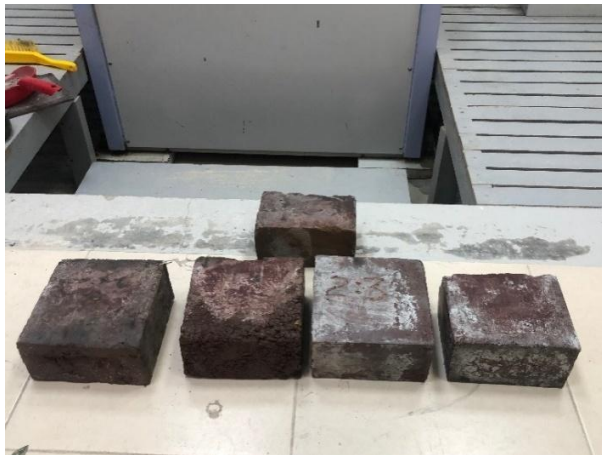
Figure 2: Manufactured Plastic Bricks Samples
