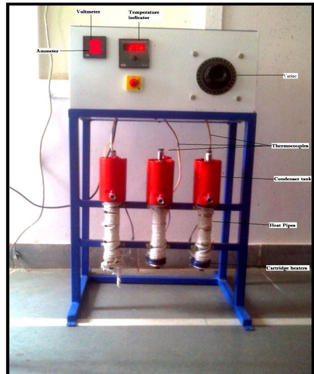
Figure no. 2: Experimental Test Rig
