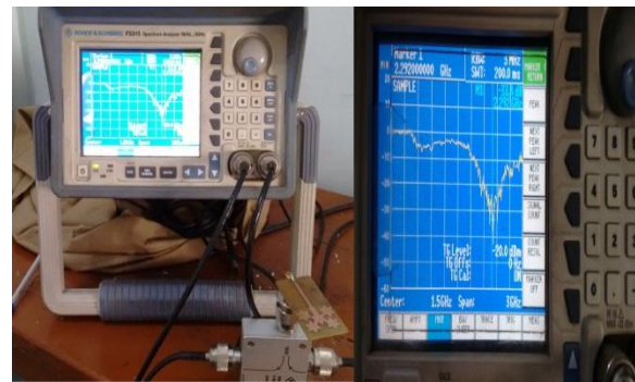
Figure 12 Measured S_{11} on spectrum analyzer.
