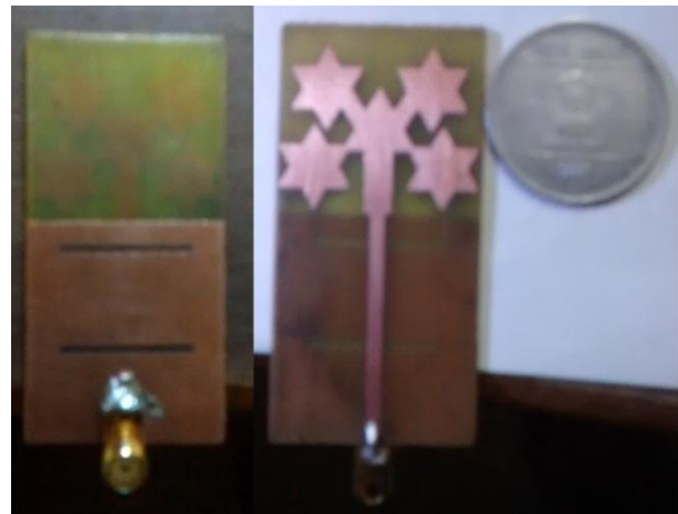
Figure (5) Fabricated antenna
