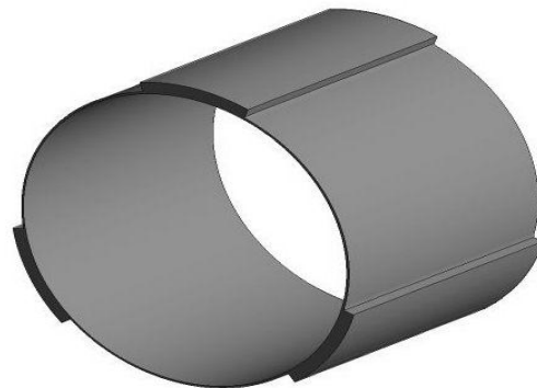
Fig 1: Schematic of 3 axial groove Journal bearing geometry
