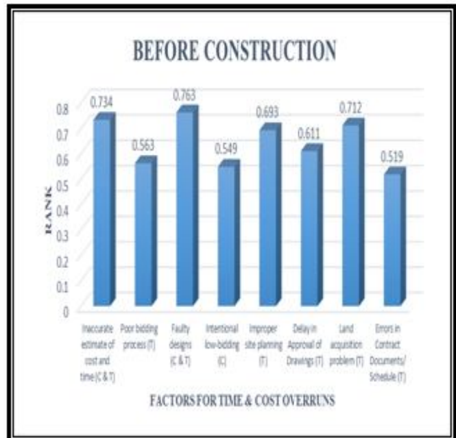
Fig 4: RII of Influencing Factors Occurs Before Construction
