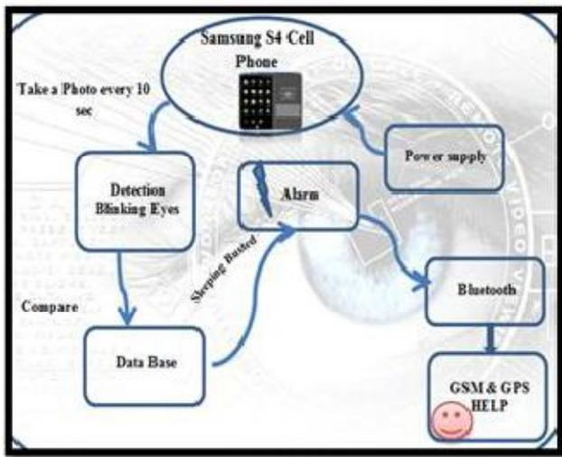
Fig 2: Block diagram of the system [3][4][5]
