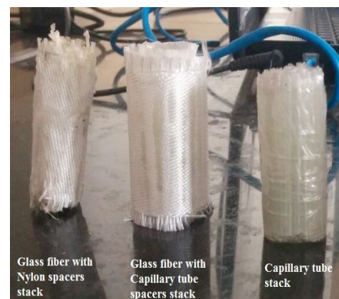
Figure 5 –Stack used for thermoacoustic experiment
