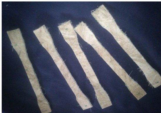
Fig. 1. Specimen prepared for tensile test
