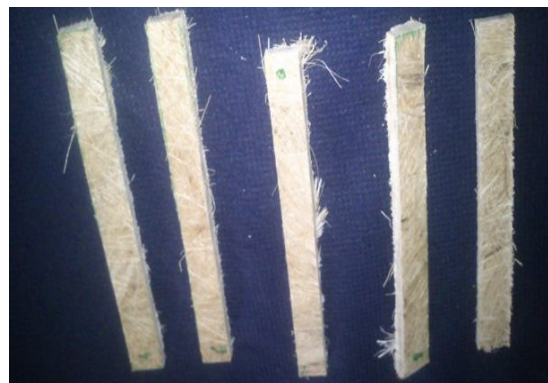
Fig. 2. Specimen prepared for flexural test
