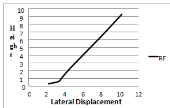
Lateral Displacement Vs Height for frame with External & Internal infill of 230mm & 115mm thick
