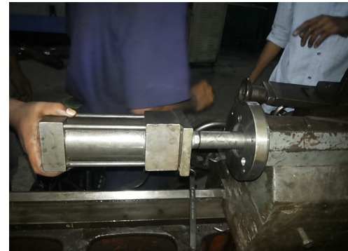
Fig. 5. Attachment of Actuator on Lathe machine
