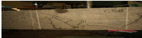
Appearance of CSB after testing
