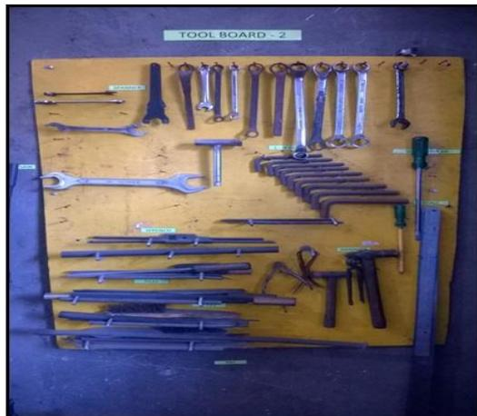
Fig 4: - Shadow board for the tools.
