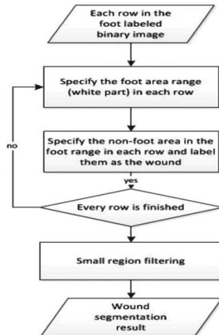
In Mean Shift Algorithm, Foot is represent as binary digit. Specify foot area as White image and binary digit as 1. Specify non foot area binary digit as other than 1. Repeat until boundary is completed. Thus wound area is determined.
