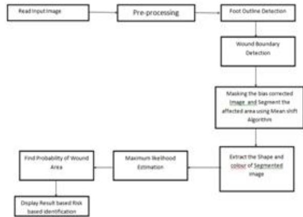
Read the input image. Remove noise while preprocessing. Determination of wound boundary using Mean shift Algorithm. Dots are noise or information that are removed. Retrieve the corrected information using Mask Bias. Use Maximum likelihood formula to extract the shape and colour. Probability of risk identification can be calculated.
