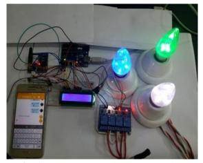
Fig -6. Actual GSM Based Home Automation
