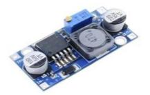
Fig 5: DC to DC Buck Converter
