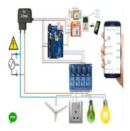
Fig -5 Block Diagram of GSM Based Home Automation
