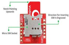
Fig 3: Sim Socket
