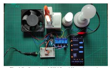
Fig -4 Configuration of GSM Based Home Automation
