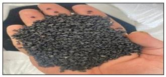
Figure 2: Waste Shredded Rubber Tyres
