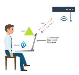
Above: Combining measurement data from a laptop's accelerometer, light sensor, gyroscope, and millimeter wave radio could enable health analytics and remote health monitoring functionality.
