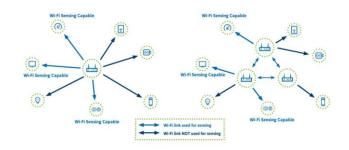
Above: An example home deployment might have one access point or multiple APs in a mesh configuration.
