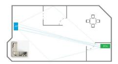
Figure 3. A representation of Multipathtransmission using MIMO
