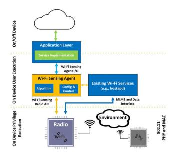
Above: A typical Wi-Fi sensing system comprises three main components: a Wi-Fi radio, a software agent for signal processing, and an application layer that turns context-aware information into services/features.
