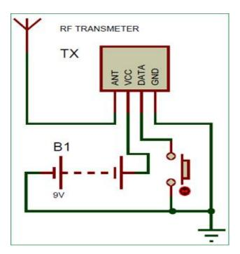
We have used a small hack to make this RF remote control circuit to work. Normally while using this 433 MHz module requires an Encoder and Decoder or two MCU to work.But, in our application we just need the receiver to detect if the transmitter is sending some signals. So the Data pin of the transmitter is connected to Ground or Vcc of the supply.
