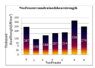
Fig4.4:% of waste vs maximum undrained shear strength.
