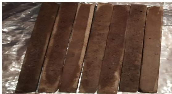
Figure 6: Plate of finished brake pad samples
