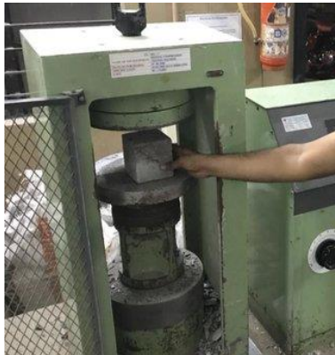
Specimen under Compressive testing Machine
