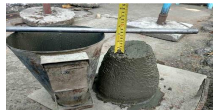
Slump Cone Test
