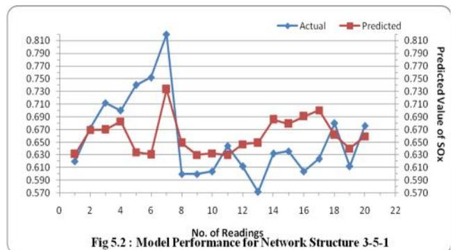
Above figure shows the performance of network with three neurons in input layer variables including temperature, humidity and wind pressure while taking  $SO_x$  as output in which maximum actual error was found to be 0.82 while minimum actual error was 0.60 whereas the maximum predicted error was 0.733 while minimum predicted error was 0.63.
