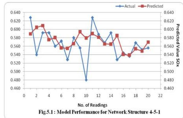
Above figure shows the exhibition of organization with four neurons in input layer factors including temperature, mugginess, wind weight and precipitation while taking Sox as yield in which greatest real blunder was discovered to be 0.62 while least real mistake was 0.48 though the most extreme anticipated mistake was 0.609 while least anticipated mistake was 0.53.
