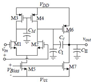
Figure 3: Miller compensated two stage op amp
