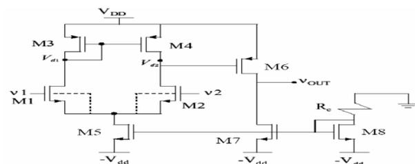
**Figure 1: Block diagram for practical operational amplifier**
