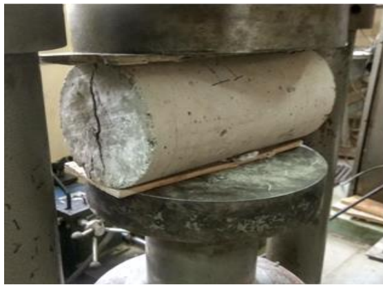
Fig 3.2: Split Tensile Testing
