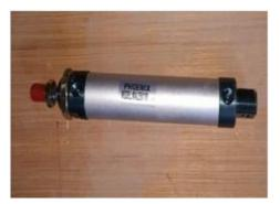
Fig : Pneumatic cylinder ( Double Acting)
