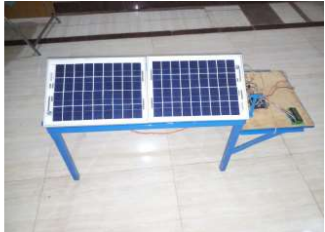
Figure 1 the Experimental setup with two solar panels with and without PCM cooling.
