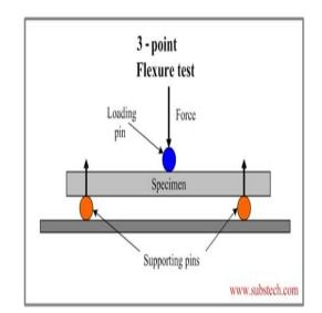
Fig. 4 3-Point Bending Test Setup
