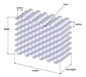
Fig. 2 Honeycomb Structure
