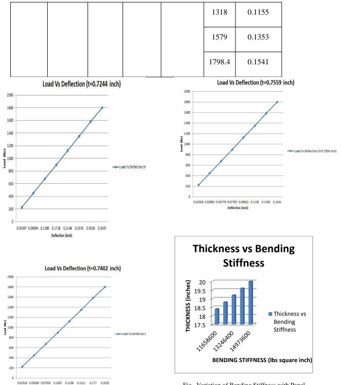
Fig. Variation of Bending Stiffness with Panel Thickness
