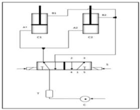
Fig.. Pneumatic Circuit
