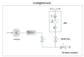
Fig..Layout of basic pneumatic system
