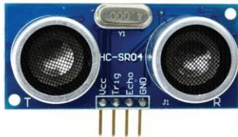
Fig 4: Ultrasonic Sensor Module
