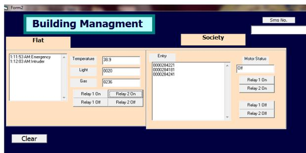
**Fig. 5: Snapshot of Building management system**
