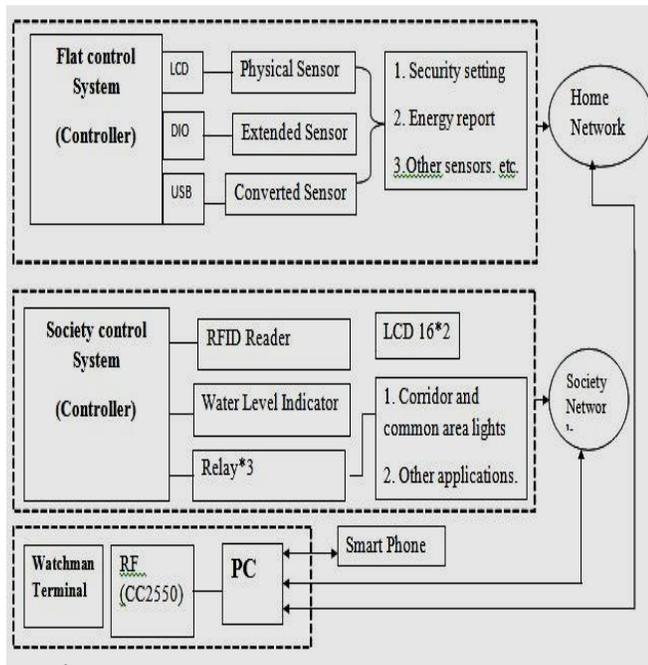
Fig. 1 shows the architecture of Flat and Society control system
