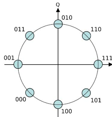
Fig 9: Constellation diagram of 8-PSK
