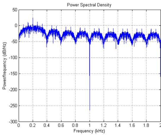
Fig 15: Energy Detector Output at SNR 30dB for 8PSK when primary user is present at 200HZ
