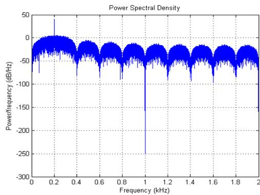
Fig 21: Energy Detector Output at SNR 30dB for 8PSK when primary user is present at 200HZ
