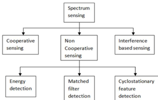
Fig 5: Classification of Spectrum sensing techniques
