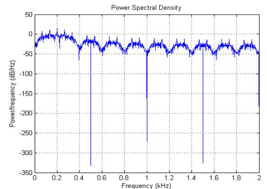
Fig 13: Energy Detector Output at SNR 30dB for QPSK when primary user is present at 200HZ
