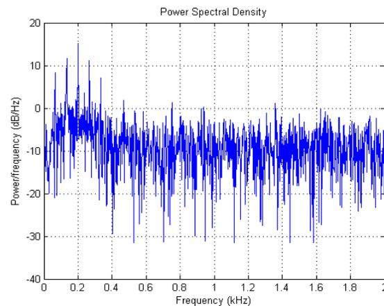
Fig 14: Energy Detector Output at SNR -30dB for QPSK when primary user is present at 200HZ
