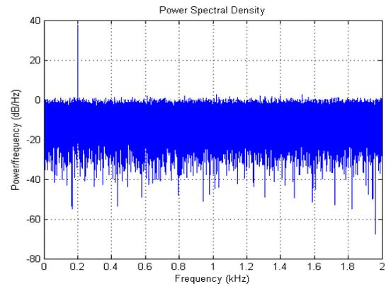
Fig 12: Energy Detector Output at SNR -30dB for BPSK when primary user is present at 200HZ
