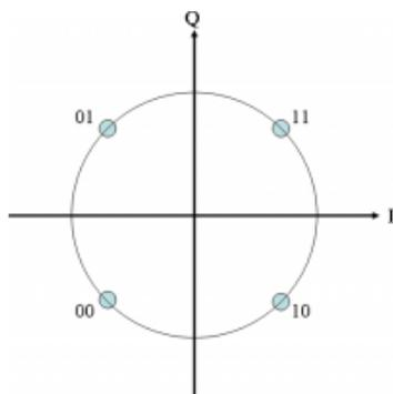
Fig 8: Constellation diagram of QPSK
