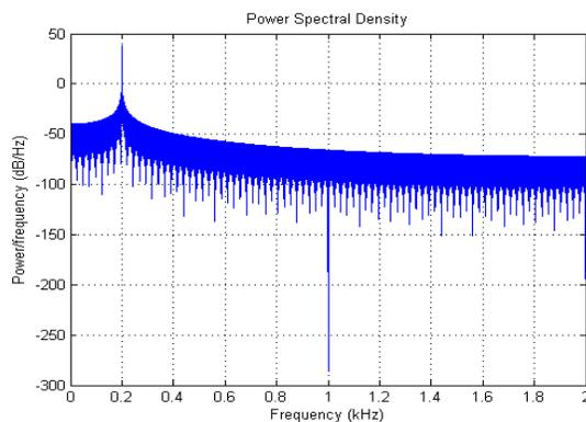
Fig 11: Energy Detector Output at SNR 30dB for BPSK when primary user is present at 200HZ
