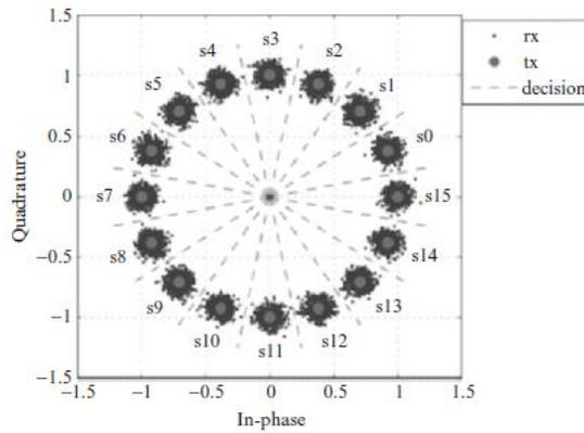
Fig 10: Constellation diagram of 16-PSK
