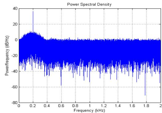
Fig 20: Energy Detector Output at SNR -30dB for QPSK when primary user is present at 200HZ
