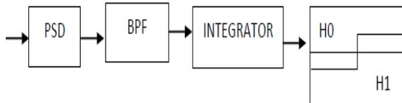
Fig 6: Block diagram of Energy detection technique
