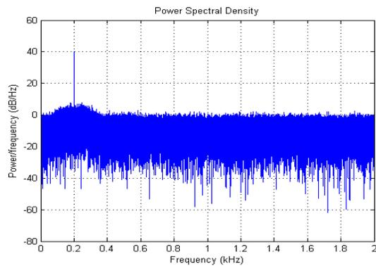
Fig 22: Energy Detector Output at SNR -30dB for 8PSK when primary user is present at 200HZ
