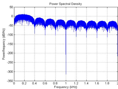
Fig 17: Energy Detector Output at SNR 30dB for BPSK when primary user is present at 200HZ
