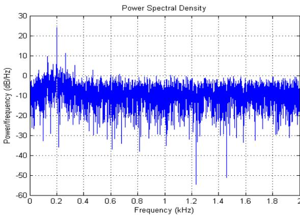
Fig 16: Energy Detector Output at SNR -30dB for 8PSK when primary user is present at 200HZ
