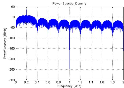
Fig 19: Energy Detector Output at SNR 30dB for QPSK when primary user is present at 200HZ
