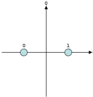
Fig 7: Constellation diagram of BPSK
