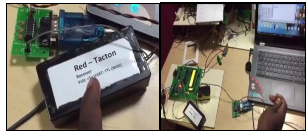
Figure. 5. Display of parameters using Red-tacton transceiver in PC
