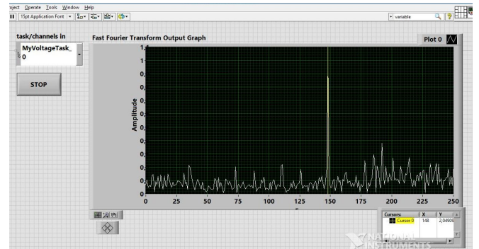
Figure 8. FFT of slower real time signal
