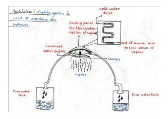
• **Canopy-** It is used to collect the vapour released during evaporation of sea water. It traps all vapour to the cooling system.
