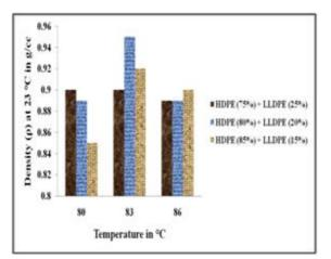
Fig. 13 Density tests result for recycled combined HDPE-LLDPE by wt%
