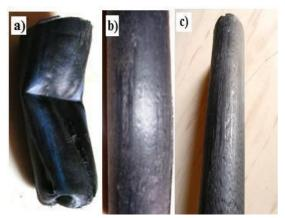
Fig. 8 Bad pipe profiles Extruded at 80°C
