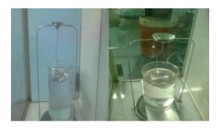
Fig. 11 Displacement method test for measuring the Density
