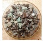
Fig. 2 Combined Recycled Granules of HDPE and LLDPE Pipe Materials
