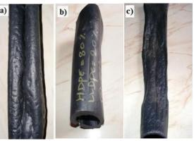
Fig. 10 Bad pipe profiles Extruded at 86°C
