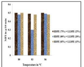
Fig. 12 MFI tests result for recycled combined HDPE-LLDPE by wt%
