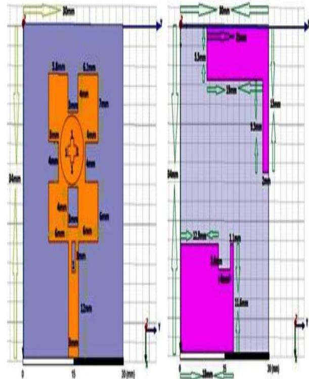
Figure 2: Proposed antenna (Top View) Figure 3: Proposed antenna (Ground View)
