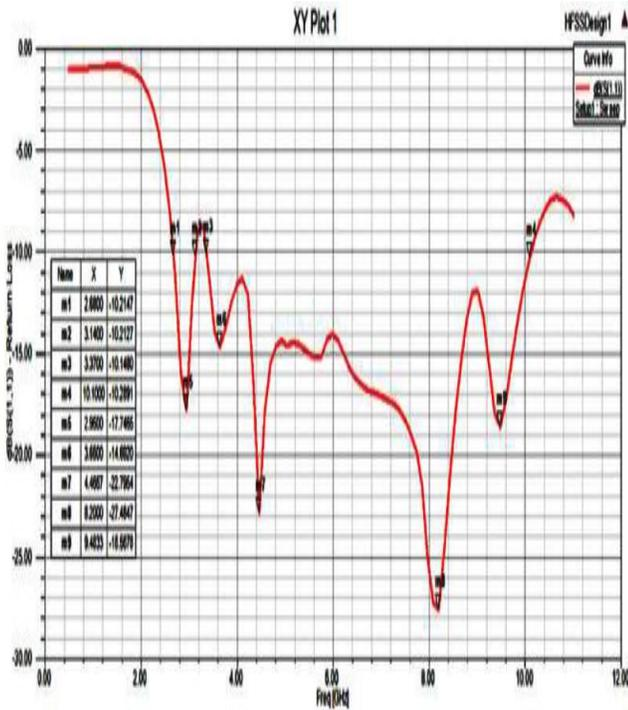
Figure 3: Plot of Simulated Return Loss(dB) vs Frequency(GHz)
