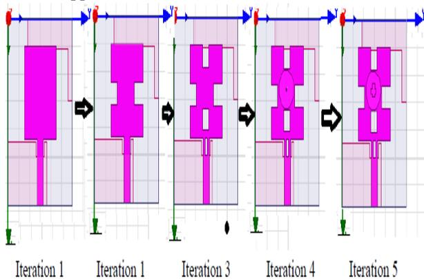
Figure 1: Successive iterations to design proposed antenna
