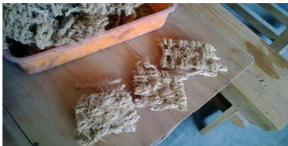
**Figure 2:** Raw coconut fibre obtained from mattress waste
