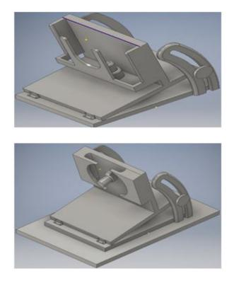
Figure shows proposed CAD model. The construction consists of clamp to hold the work piece horizontally from both the end and projection used to centered the work piece. Autocad Inventor is used as design software for fixture. The plane is provided to rotate the work piece with the help of scale which is located at the both sides of the plane.
