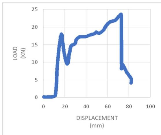
Fig 10:- Load vs displacement curve of shore 70 elastomer filled aluminium tube
