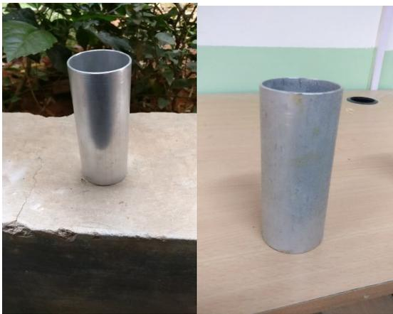
Fig 1:- Non annealed and annealed aluminium tube
