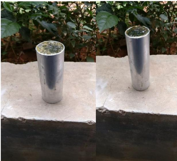
Fig 2:- Polyester and vinyl ester filled annealed aluminium tube.
