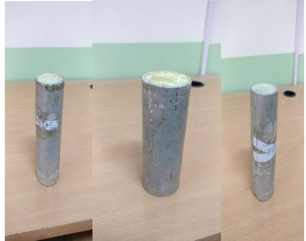
Fig 3:- Shore 45, 60 and 70 Elastomer filled annealed aluminium tube.
