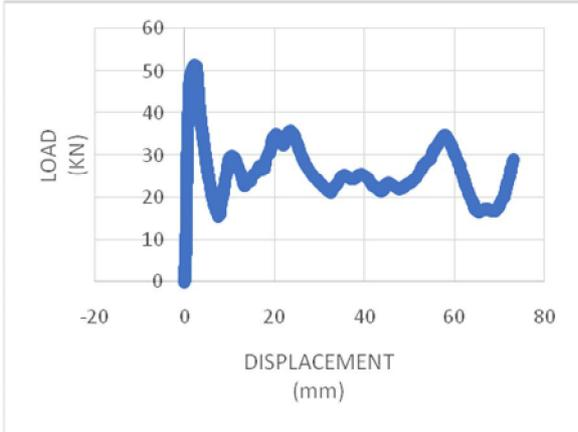
Fig 4:- Load vs displacement curve of Non Annealed empty aluminium tube
