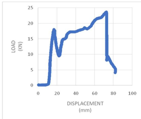
Fig 10:- Load vs displacement curve of shore 70 elastomer filled aluminium tube
