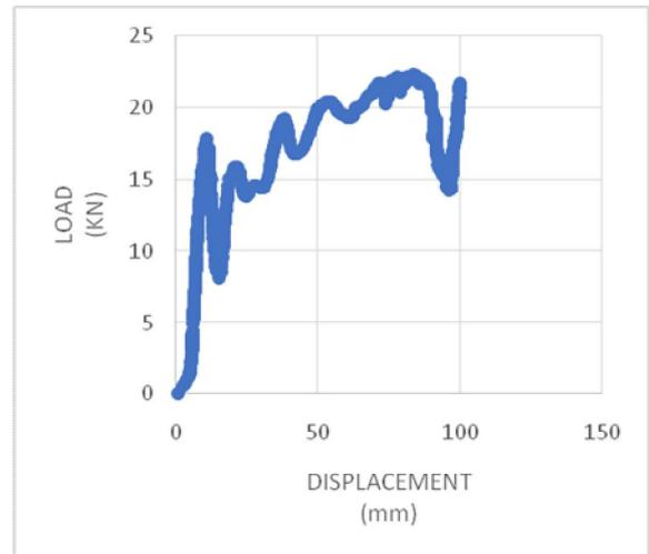
Fig 9:- Load vs displacement curve of shore 60 elastomer filled aluminium tube
