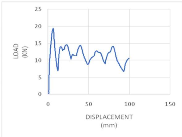
Fig 5:- Load vs displacement curve of Annealed empty aluminium tube
