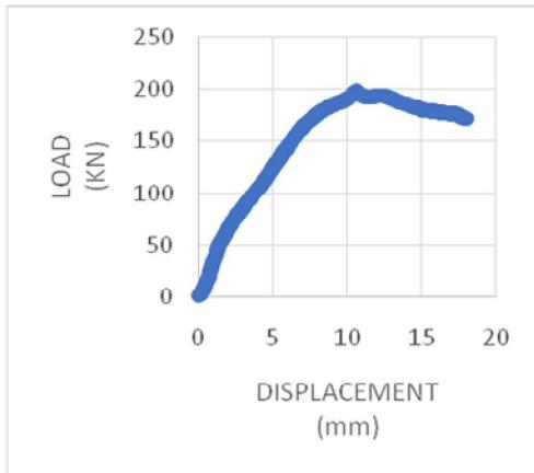
Fig 6:- Load vs displacement curve of vinyl ester filled aluminium tube
