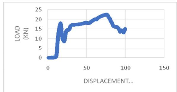
Fig 8:- Load vs displacement curve of shore 45 elastomer filled aluminium tube
