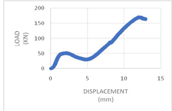
Fig 7:- Load vs displacement curve of polyester filled aluminium tube
